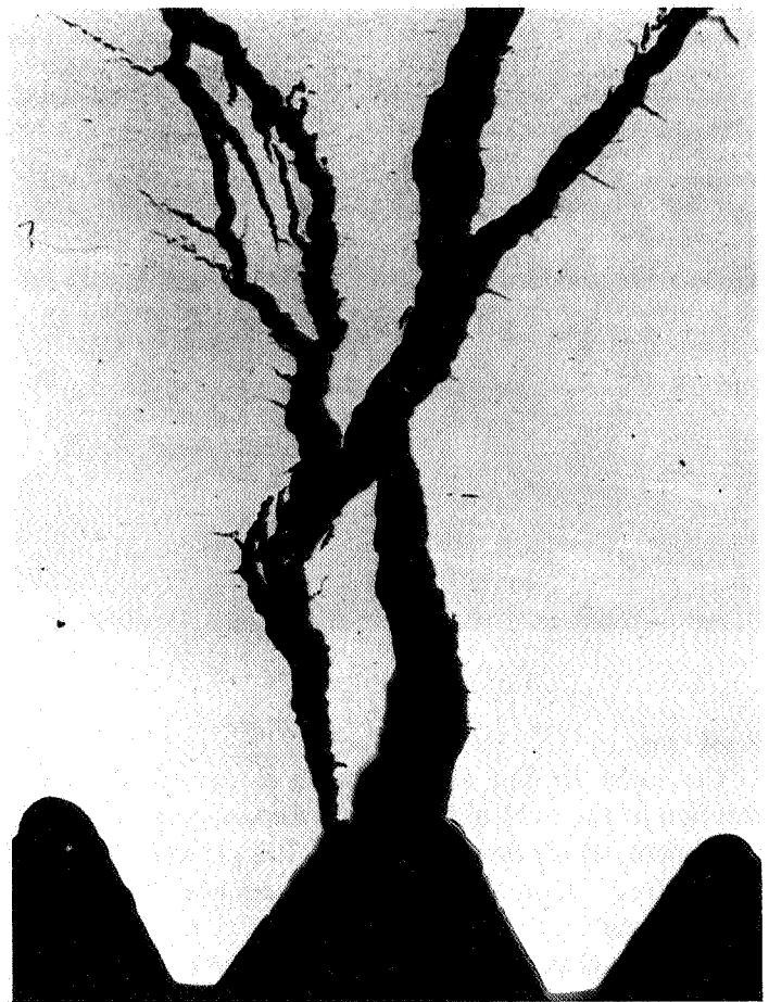
Figure 5. Photomicrograph illustrating branching cracks in the long sample (nital etch; mag: 10X).
